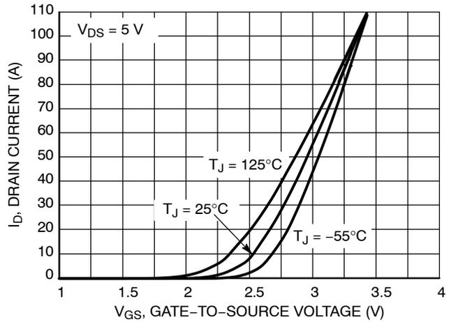
Figure 2. Transfer Characteristics
