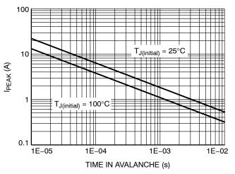
Figure 12. I<sub>PEAK</sub> vs. Time in Avalanche
