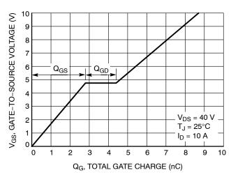
Figure 8. Gate-to-Source Voltage vs. Total Charge
