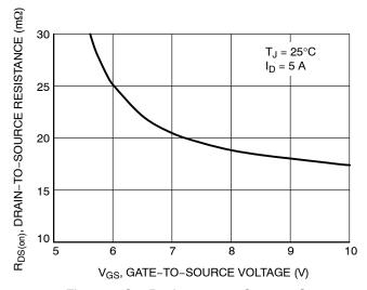
Figure 3. On-Resistance vs. Gate-to-Source Voltage
