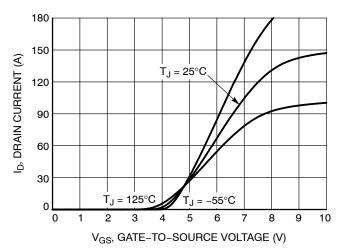
Figure 2. Transfer Characteristics
