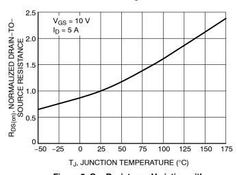
Figure 5. On–Resistance Variation with Temperature
