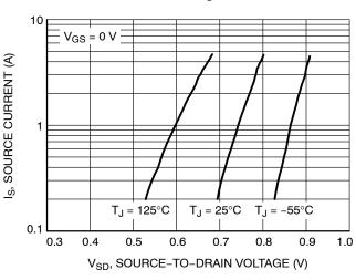
Figure 10. Diode Forward Voltage vs. Current
