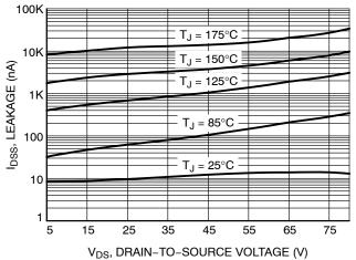
Figure 6. Drain-to-Source Leakage Current vs. Voltage
