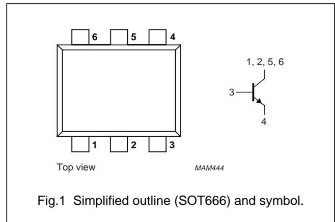
40 V low  $V_{CEsat}$  NPN transistor
