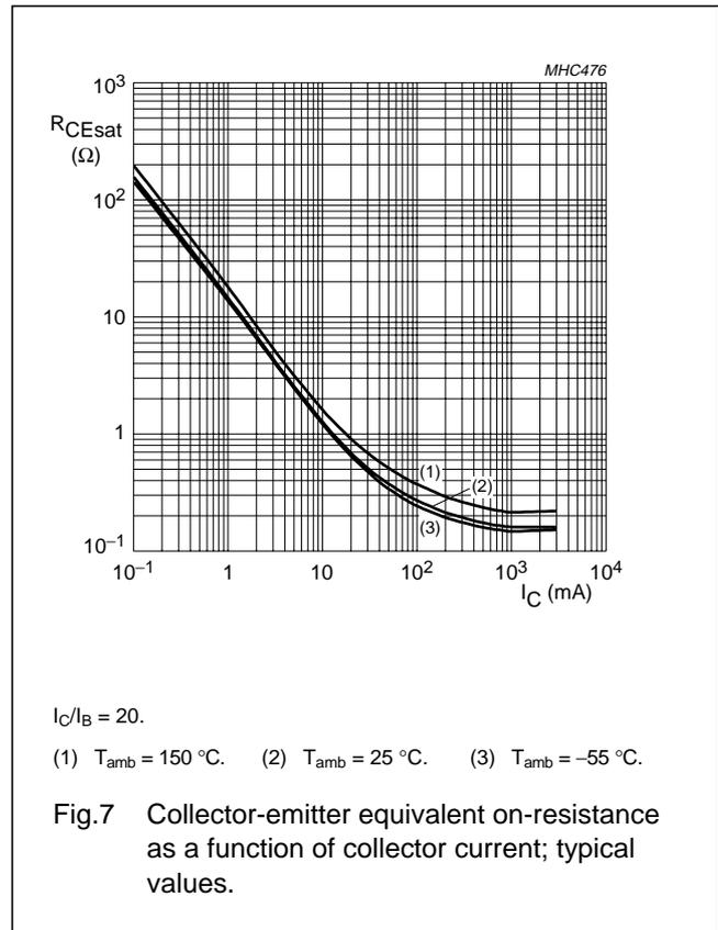
40 V low  $V_{CEsat}$  NPN transistor
