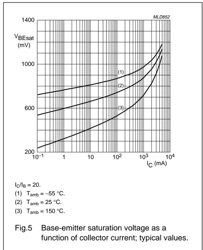
20 V low  $V_{CEsat}$  NPN transistor
