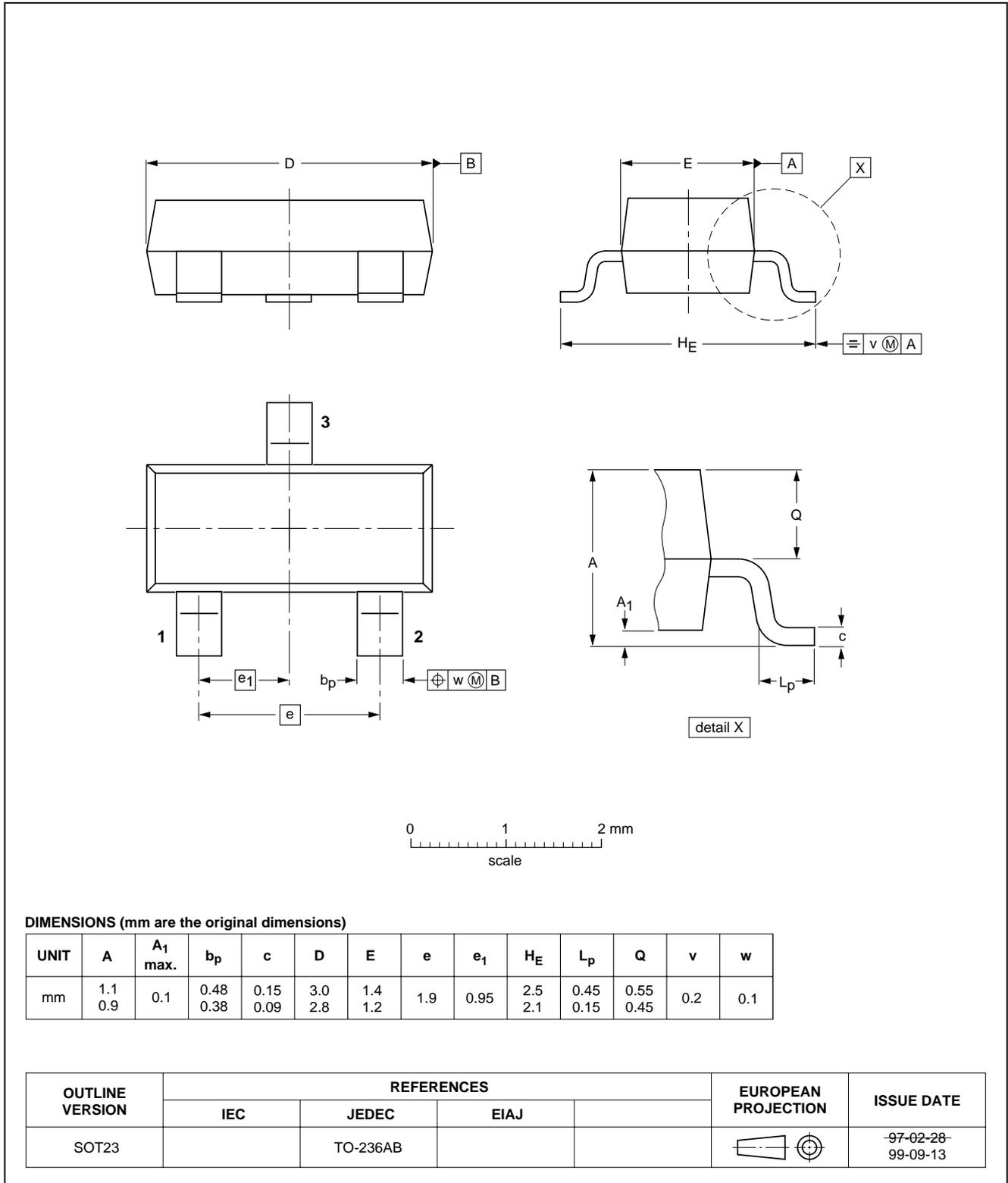
20 V low  $V_{CEsat}$  NPN transistor
