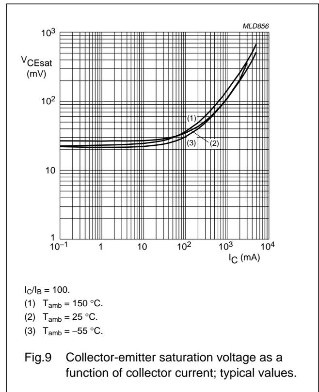
20 V low  $V_{CEsat}$  NPN transistor
