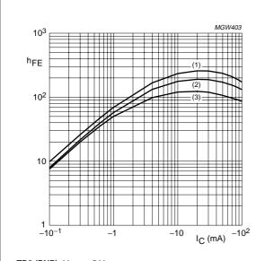
TR2 (PNP);  $V_{CE} = -5 \text{ V}.$
