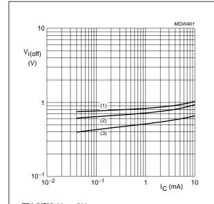
TR1 (NPN);  $V_{CE} = 5 \text{ V}.$
