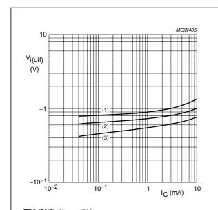
TR2 (PNP);  $V_{CE} = -5 \text{ V}.$
