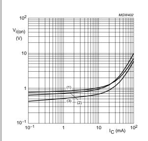
**TR1 (NPN);**  $V_{CE} = 0.3 \text{ V}.$
