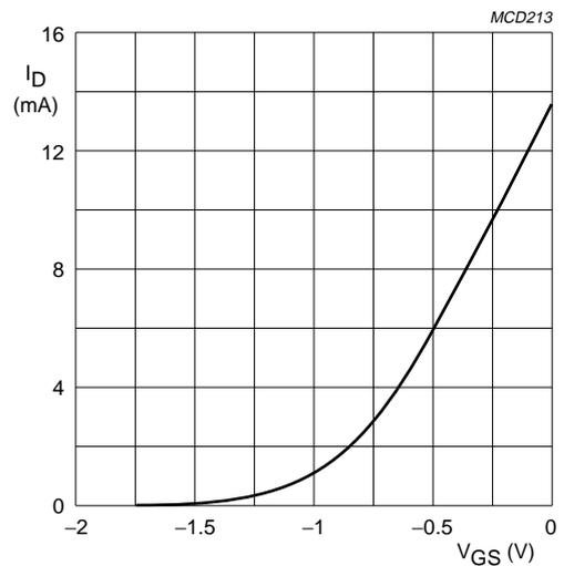
$V_{DS} = 10 \text{ V}; T_j = 25 \text{ }^\circ\text{C}.$
