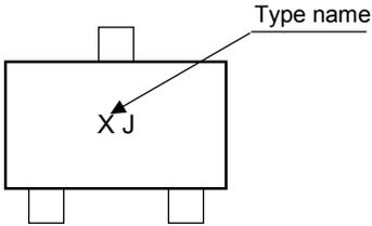
A schematic diagram of a rectangular component with a top pin and two bottom pins. The marking 'XJ' is centered on the component. An arrow labeled 'Type name' points to the 'J' in 'XJ'. |
