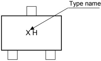
A schematic diagram of a rectangular component with a top pin and two bottom pins. The marking 'XH' is centered on the component. An arrow labeled 'Type name' points to the 'H' in 'XH'.  |
