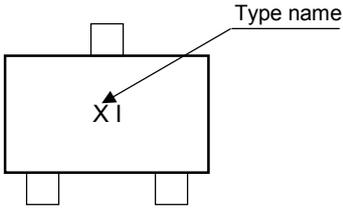
A schematic diagram of a rectangular component with a top pin and two bottom pins. The marking 'XI' is centered on the component. An arrow labeled 'Type name' points to the 'I' in 'XI'.  |
