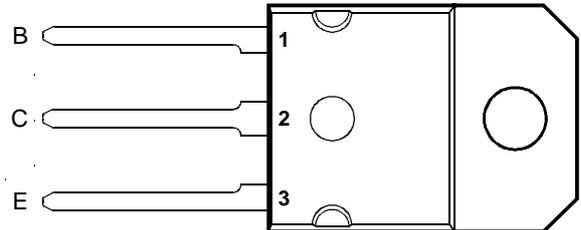
Pin 2 is in electrical contact with the mounting base.
