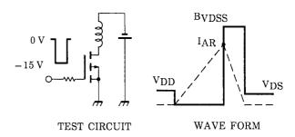
$$\begin{array}{ll} T_{ch} = 25^{\circ}C \; (\rm{Initial}) \\ Peak \; I_{AR} = -7 \; A, \; R_G = 25 \; \Omega \end{array} \quad E_{AS} = \frac{1}{2} \cdot L \cdot I^2 \cdot (\frac{B_{VDSS}}{B_{VDSS} - V_{DD}}) \\ V_{DD} = -24 \; V, \; L = 1.0 \; mH \end{array}$$
