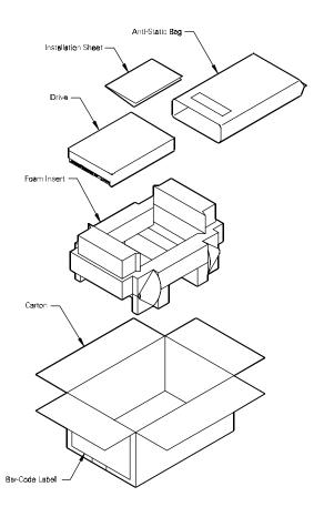
Figure 4 - 2 Single Pack Shipping Container (Option A)
