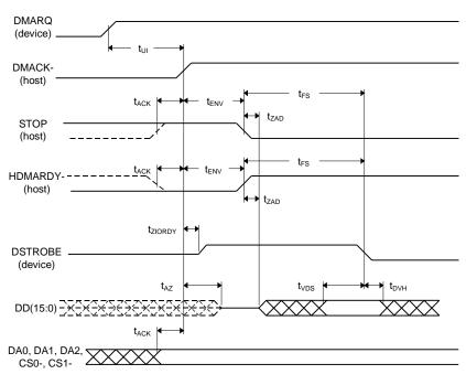
Figure 5 - 4 Initiating an Ultra DMA Data In Burst
