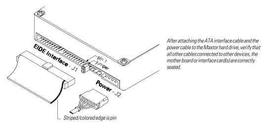
Figure 4 - 4 ATAInterface and Power Cabling
