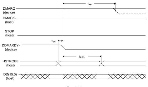
Figure 5 - 11 Device Pausing an Ultra DMA Data Out Burst
