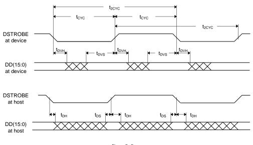
Figure 5 - 5 Sustained Ultra DMA Data In Burst
