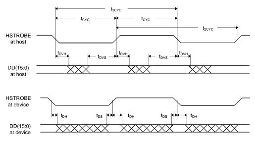
Figure 5 - 10 Sustained Ultra DMA Data Out Burst
