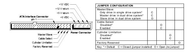
Figure 2-1 PCBA Jumper Location and Configuration
