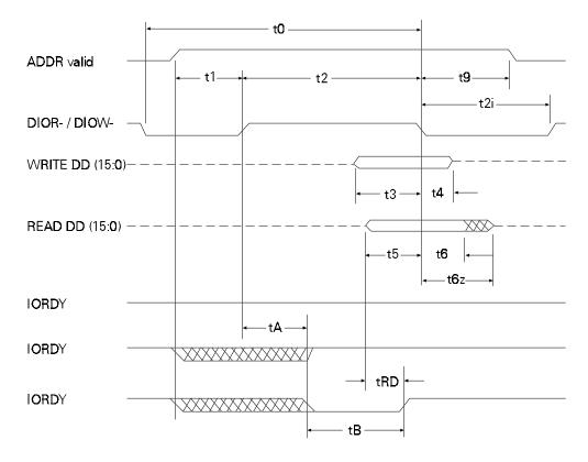
*Figure 5 - 2 PIO Data Transfer To/From Device*
