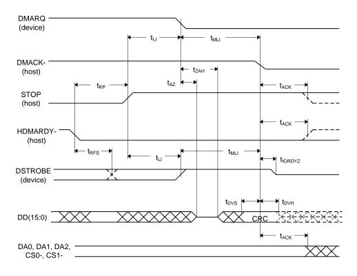
Figure 5 - 8 Host Terminating an Ultra DMA Data In Burst
