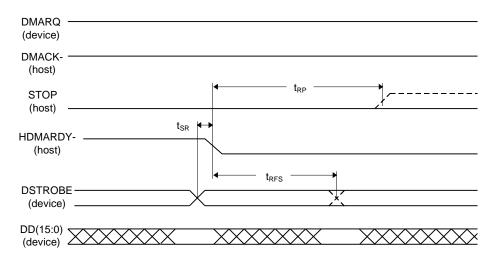
Figure 5 - 6 Host Pausing an Ultra DMA Data In Burst
